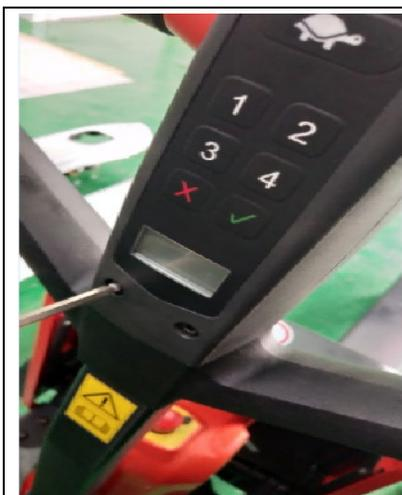
Tiller rear cover fixing bolt removed with 5mm hexagon socket
