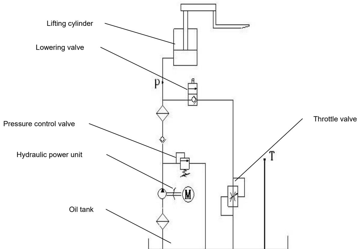
Fig.24: Hydraulic circuit
