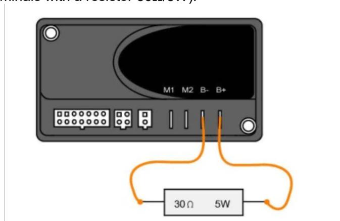
Use a multimeter to measure according to the table below and check whether it is normal. Each test item must be tested more than 3 times.
