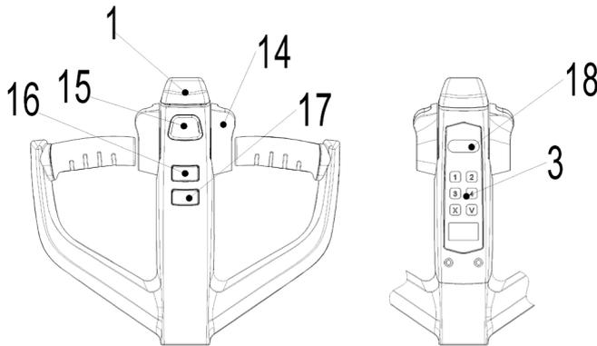
**Fig.7:** 20EP-XB control tiller
