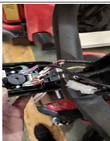
Remove the tiller back cover by unplugging the connector
