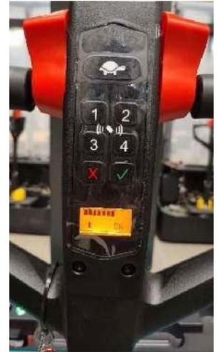
**Fig.8:** Tiller operating controls
