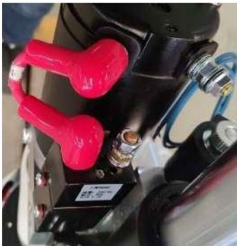
Use a 10mm open-end wrench to remove the contactor pile head cable, use a Phillips screwdriver to remove the contactor bracket fixing bolt, remove the contactor together with the bracket and then split
