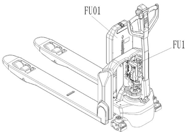
Fig. 16: Location of fuses for 20EP-XB
