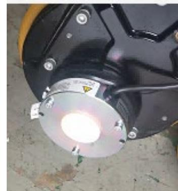
Remove the brake by removing the three brake retaining bolts with a 4mm hexagon socket.
