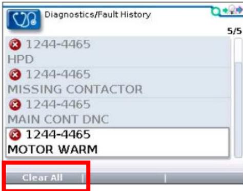
"Clear All" is used to Clear the history failure folders. A function key will be highlighted separately if there is a history failure in the history failure folder, and will be grayed out if there is no history failure.
