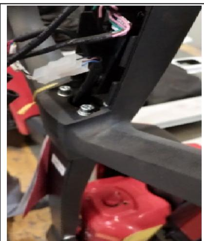
tiller front cover 4 fixed bolts can be removed with a 5mm hexagonal socket, you can remove the tiller
