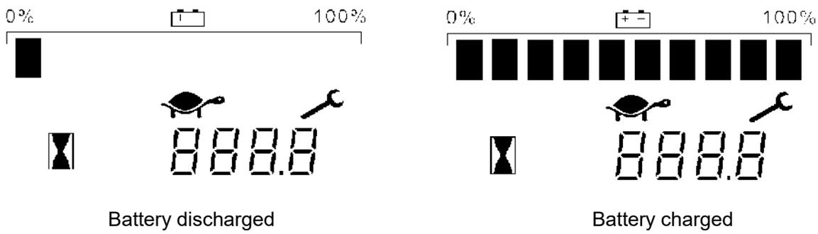
Fig. 12: Battery discharge indicator
