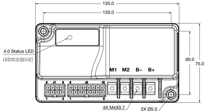
Docking connector: 8core Molex Mini-Fit Jr.
