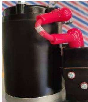
Remove the line at the contactor insert
