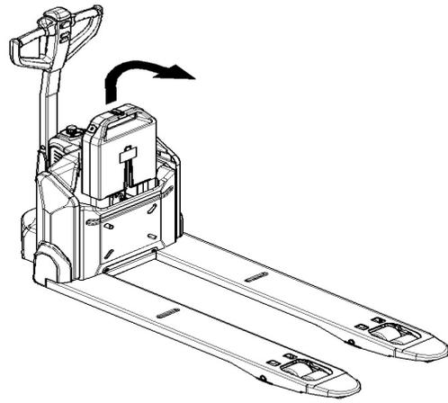
Fig.11: Replacing the battery
