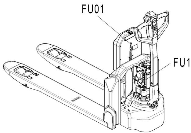
Fig. 15 Location of fuses for 15EP-XB
